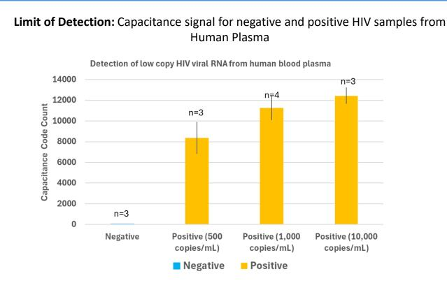
Specificity of the CMOS chip detector is demonstrated by the very low negative sensor results depicted on the graph.
