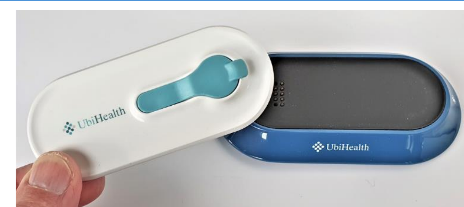
Fig. 6: Single-use disposable per test (low-cost injection-moulded) Reusable Base Reader Unit with encryption & wireless upload.
